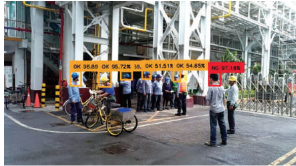
Real-time Indication of Workers Not Wearing a Helmet by the Helmet Detecting System
