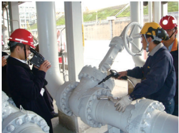
Infrared Gas Display Device for Finding Unobvious Leaks
